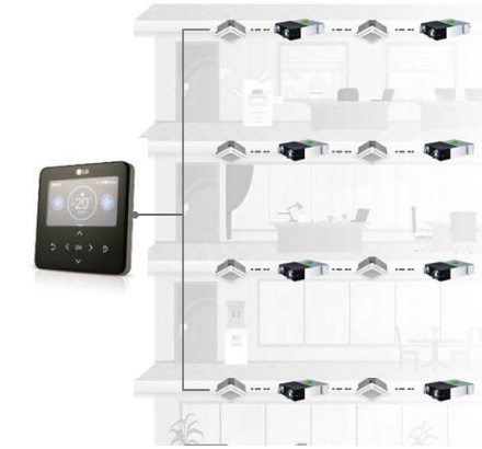
1) 16 units (including ERV, air conditioner) + 1 remote controller
